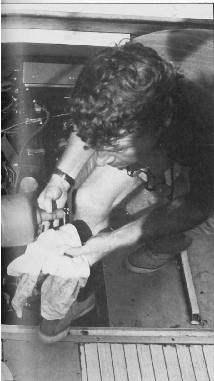
Although the diesel engine was never shut down, Cargile carefully checked fuel filters and oil level daily
