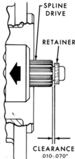
Figure 27—Checking pinion clearance on spline drive motor.
