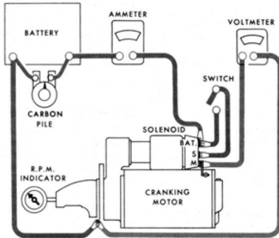
Figure 9—No-load test circuit.
