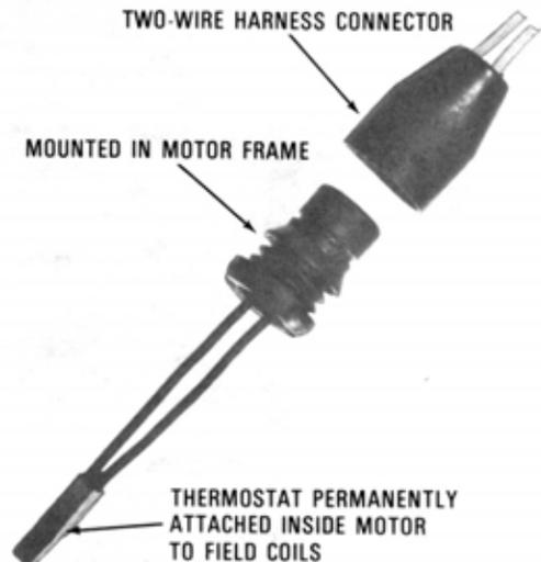
Figure 7—Typical thermostat.
