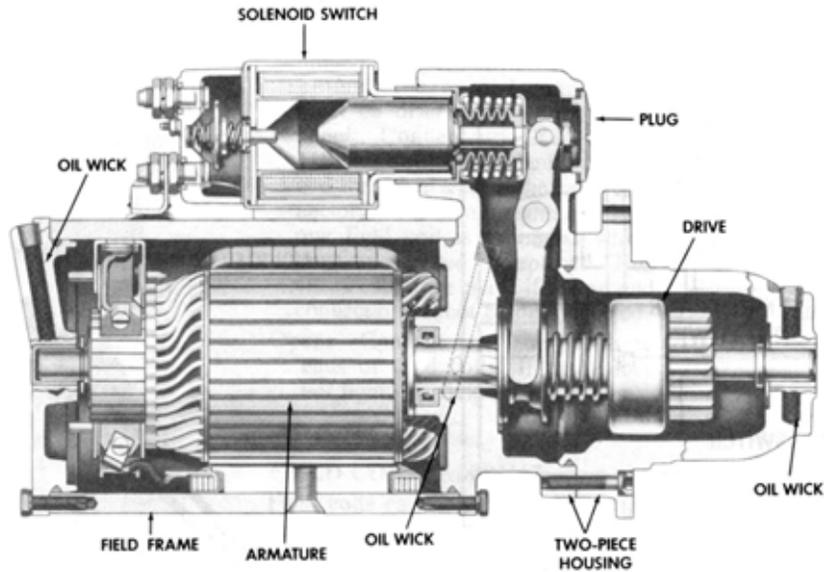
Figure 4—Cross-sectional view of motor with intermediate duty clutch. (35-MT) Note different attaching bolt construction than Figure 5.
