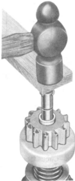
Figure 20—Forcing snap ring over shaft.
