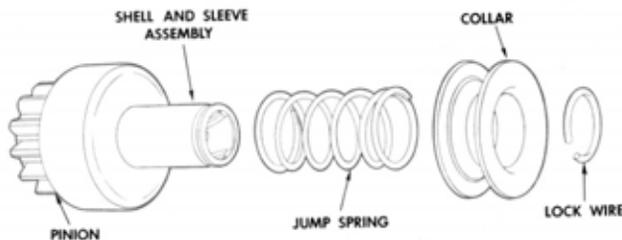
Figure 13—Disassembled view of late type intermediate duty sprag clutch drive assembly.
