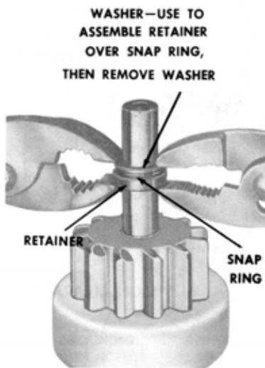
Figure 21—Forcing retainer over snap ring.
