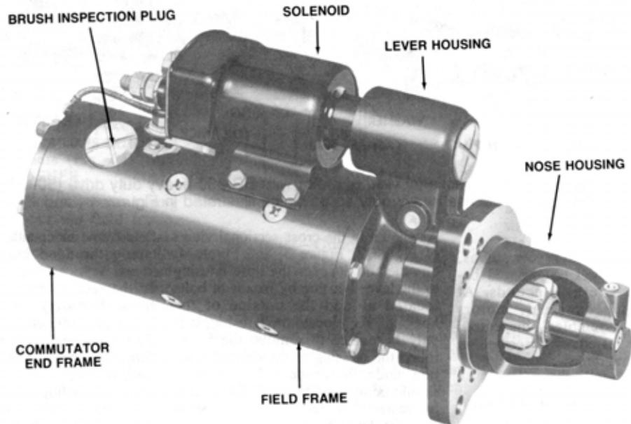
Figure 1—Typical 50-MT Series heavy duty cranking motor.
