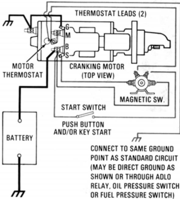
Figure 6—Basic wiring circuit.
