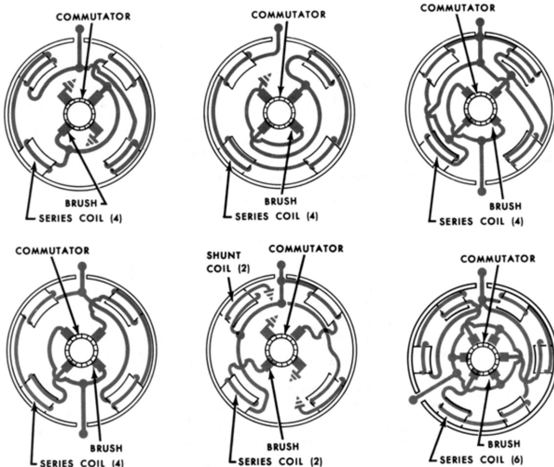
Figure 11—Typical motor circuits.
