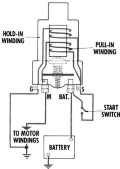
Figure 17—Basic solenoid circuit. (Types shown in Figures 1, 2, and 3.)
