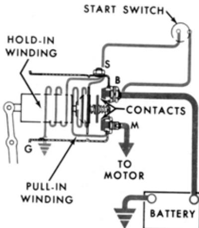
Figure 18—Basic solenoid circuit. (Types shown in Figures 4 and 5.)
