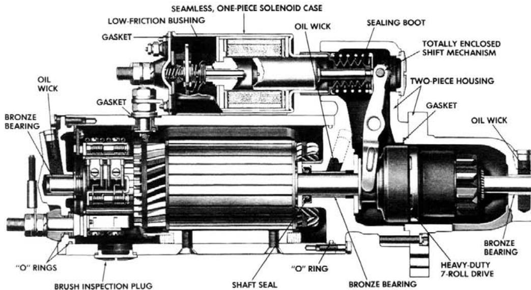
Figure 2—Cross-sectional view
