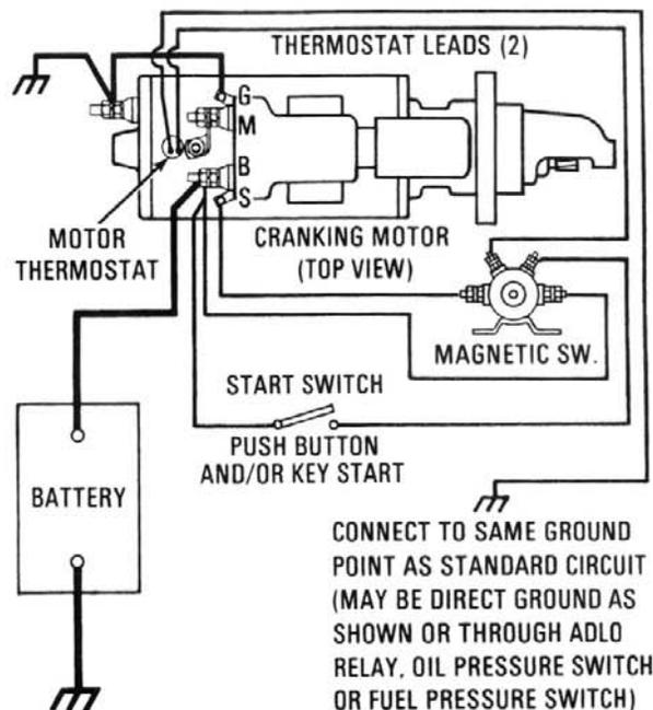
Figure 3—Typical wiring circuit
