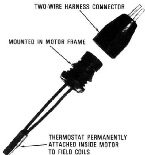
Figure 4—Typical thermostat
