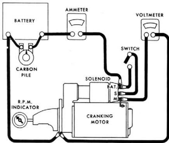
Figure 6—No-load test circuit
