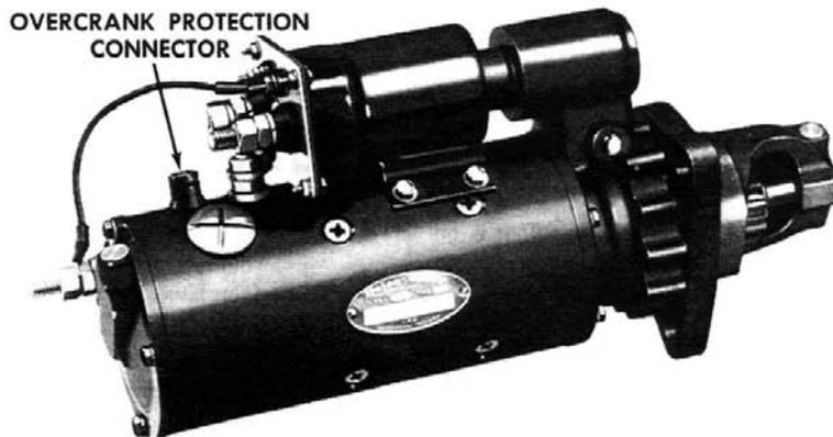
Figure 5—Typical motor showing thermostat connector (Overcrank Protection Connector)
