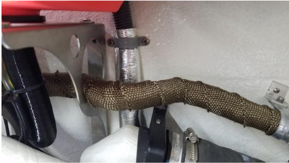
Exhaust Pipe Exit Routing
