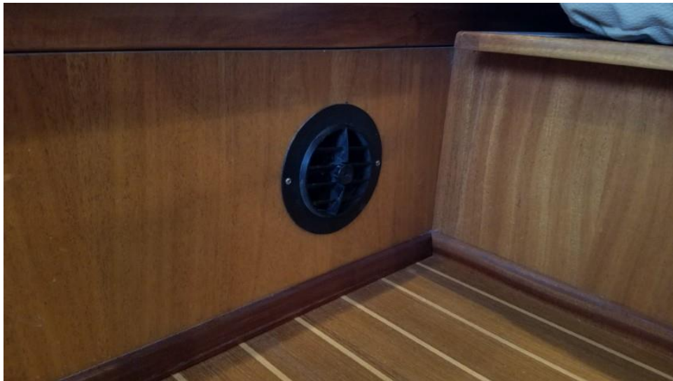
Fresh Air Intake Under Aft Salon Seat
