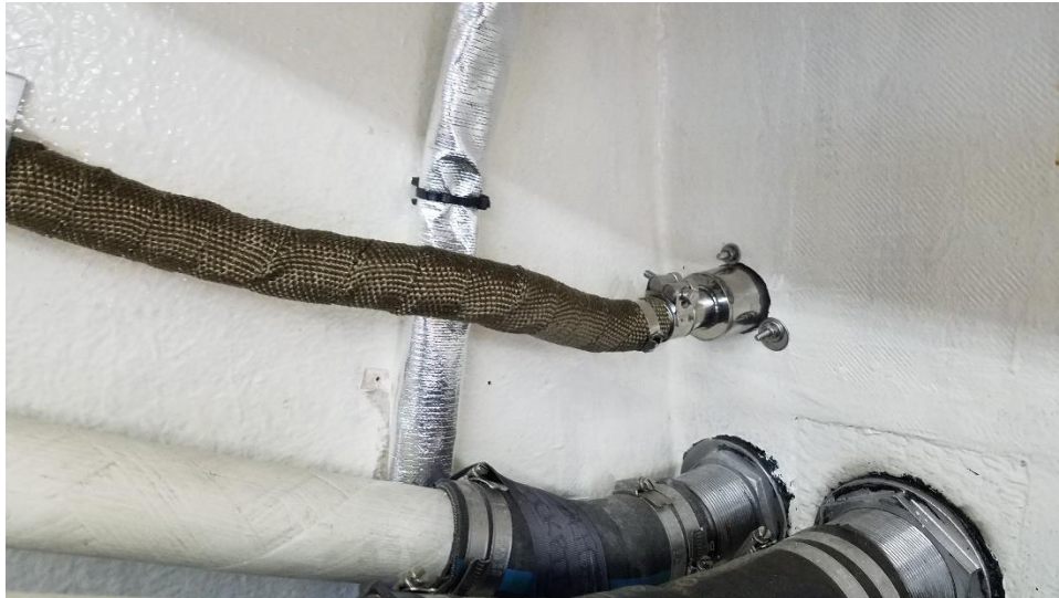
Exhaust Pipe Routing and New Thru Hull
