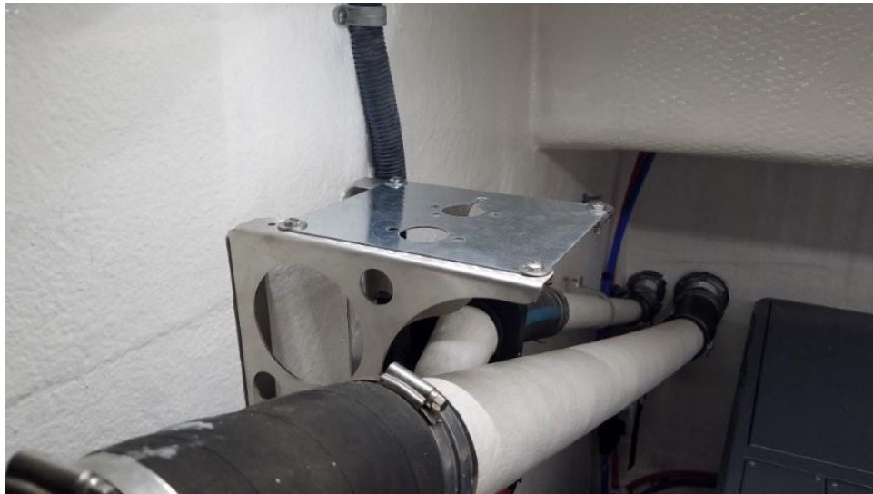
Allowing for the Exhaust Run to the Thru Hull
