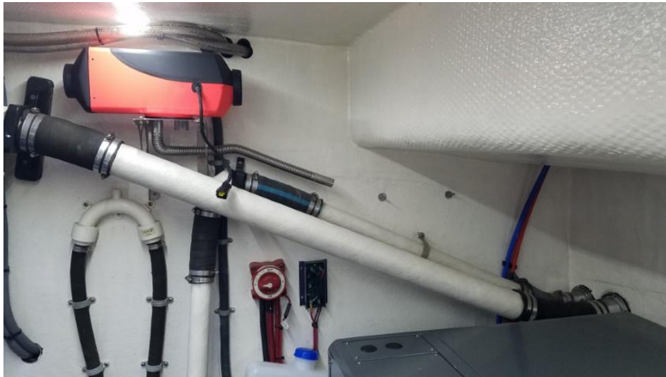
Testing Heater Mount and Exhaust Hose Routing
