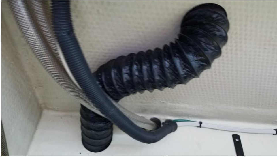
Fresh Air Intake Duct Through Bosun's Locker Up To Salon Seat
