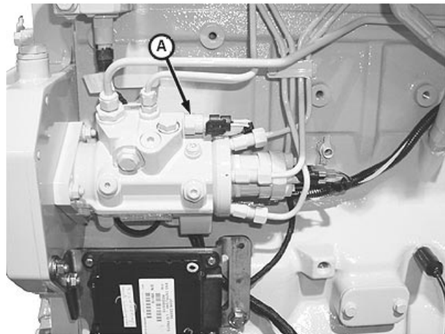
Fuel Temperature Sensor
