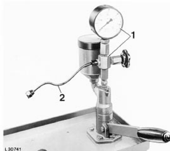
Fuel Injection Nozzle Test
