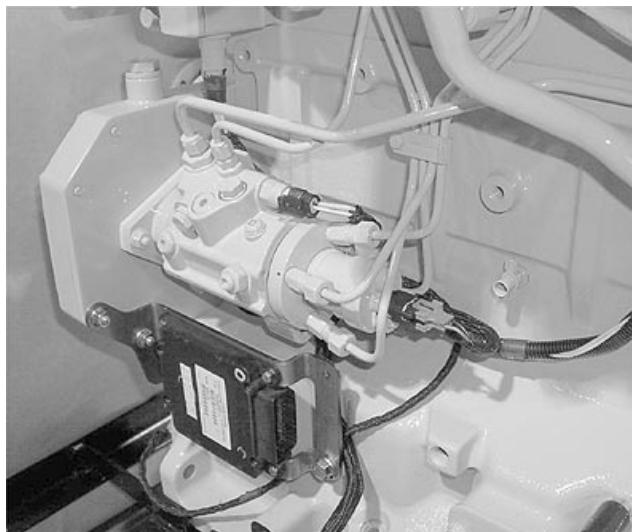
Stanadyne DE10 Fuel Injection Pump
