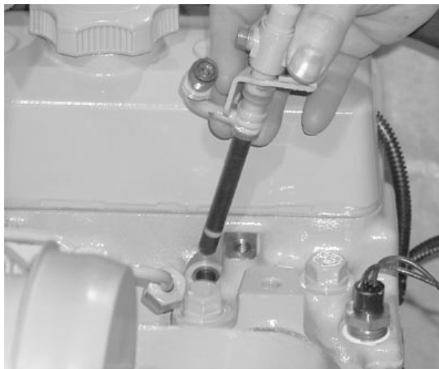
Injection Nozzle in Cylinder Head
