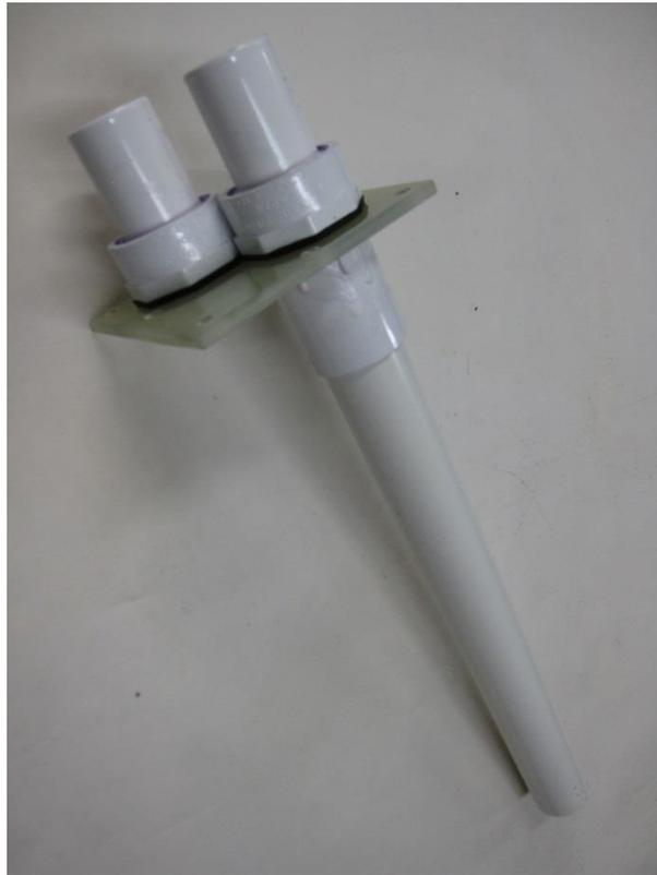
All that remained to return the holding tank to functionality was to bolt the plate assembly to the top of the tank (using the new rubber gasket I made) and re-attach to inlet and discharge hoses. A little trimming of the hoses was required since the hose adapters are slightly longer than the original copper pipes.
