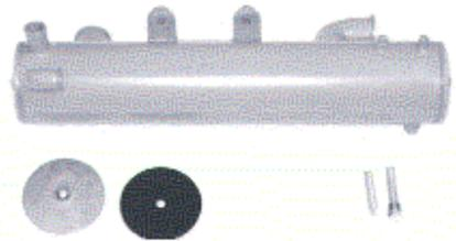
**Exhaust Elbow.** Replace the exhaust elbow before the bottom blows out as shown on the attached photo. The standard 810-0371 Lehman 120 elbow has a 3.5" O.D. hose bib for attachment of the exhaust hose. Lehman 80 engines used the 810-0372 Elbow supplied with a 3" O.D. hose bib. It is OK to use the 3.5" on a four cylinder. Some installations require the 810-0283, 3" female pipe thread elbow for installation of a 90 degree sweep fitting.
