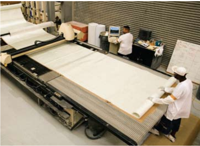
CNC laser accurately cuts roving for the hull sides.
