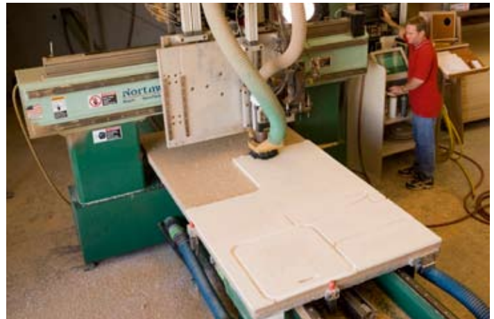
The computer-controlled cutter cuts panels with tremendous accuracy for tight fit-ups.
