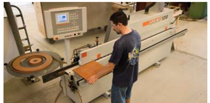
The computer-controlled edger provides a quality finish for the cabinet door.
