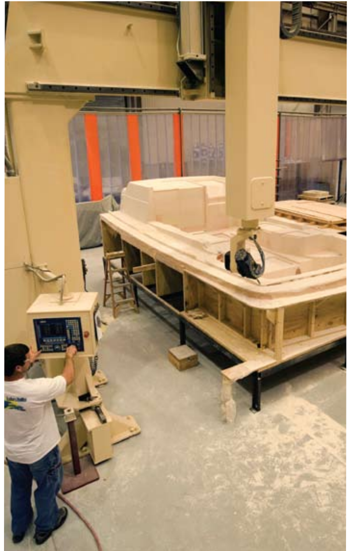
Highly sophisticated Five-Axis Router creating the plug for a deck mold.
