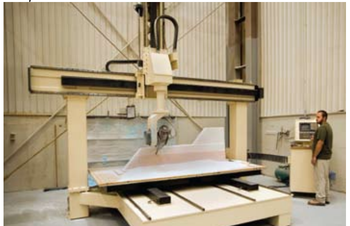
CNC controlled router creating the plug for fiberglass hull component.
