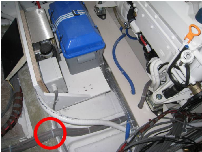
Figure 3: Cutting place of negative engine cable.
