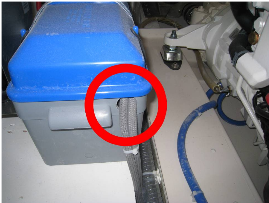
Figure 6: Engine battery (#201) and VW engine connections connected together to negative pole of engine battery.
