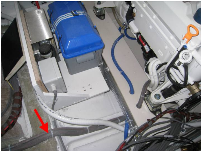
Figure 2: Main harness of VW engine.
