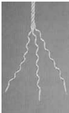
2. Pass the outer strands down through the link. Pass the inner strand up through the link and tuck back under itself.
