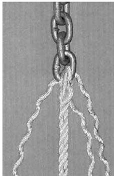
3. Once finished splicing, cut and seal the ends of the strands with a hot knife.
