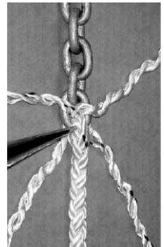
3. Once finished splicing, cut and seal the ends of the strands with a hot knife.
