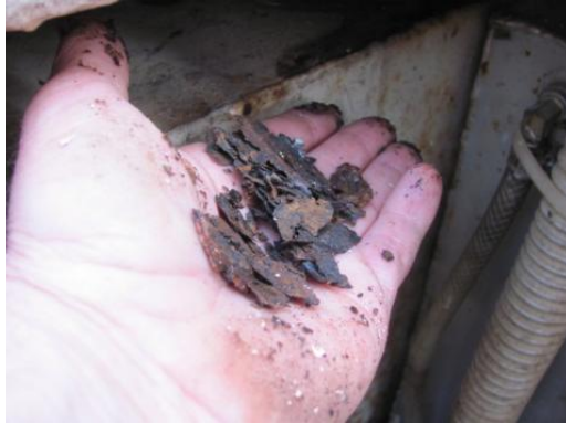
Corrosion from top of starboard tank
