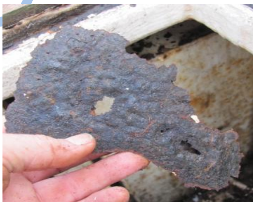
Corrosion peeled from top of port tank
