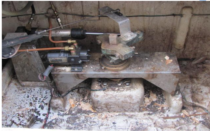
Hydraulic steering gear
