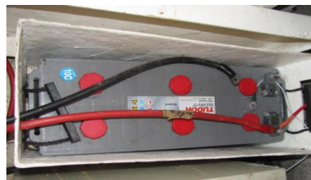
No box, no fuse, no terminal protection
