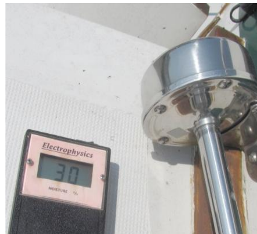
Pilot house deckhead -high moisture
