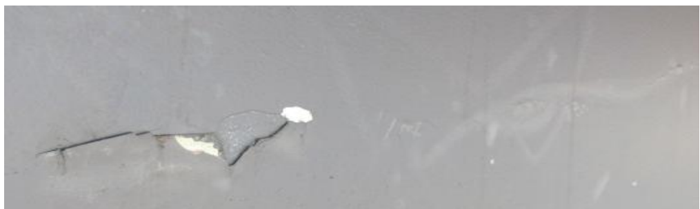
Flaking gelcoat on keel to starboard
