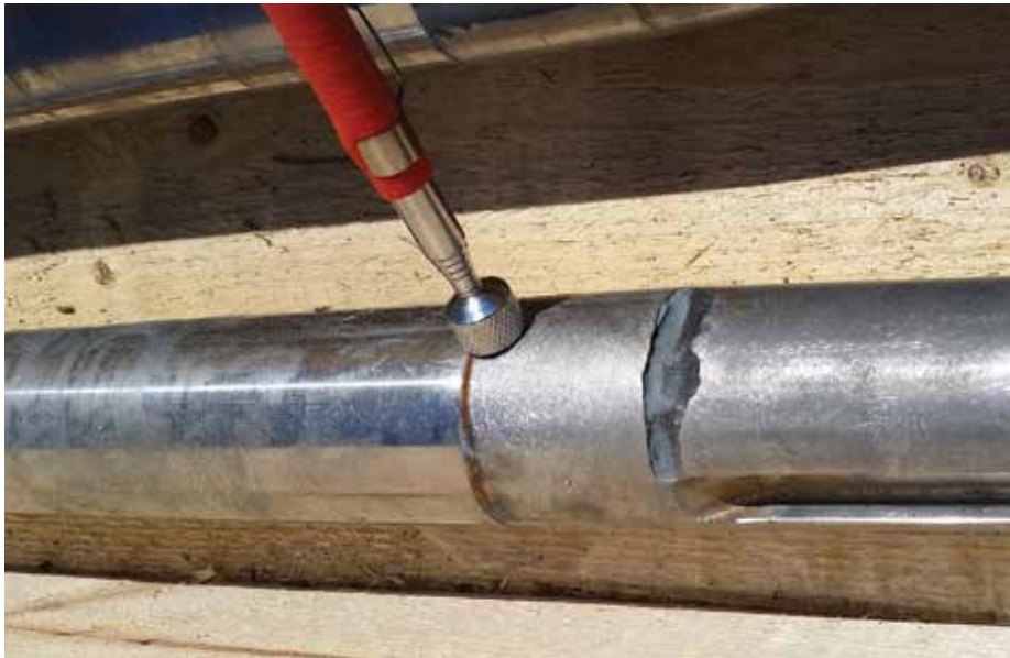
Only lower-grade alloys will attract a magnet. Severe crevice corrosion has developed at the forward end of the keyway area.
