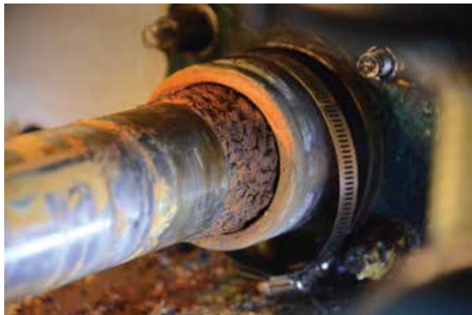
Low-grade alloy immersed in an oxygen-starved environment does not hold up well. Severe scaling and corrosion have destroyed this shaft in the seal area.
