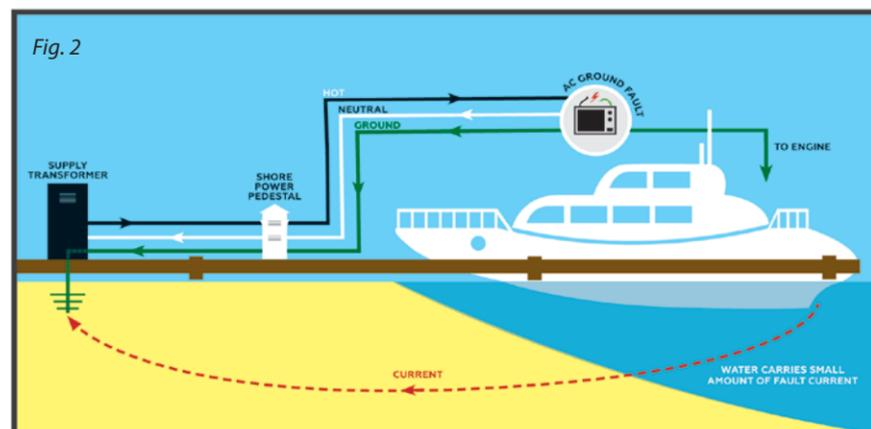
we can see that the hot and neutral wires bring shore power to the appliances. The green wire is on "standby," with no current flowing through it. If current does flow in the green wire, a "ground fault" has occurred. We'll explain that green wire to the engine in a moment.
