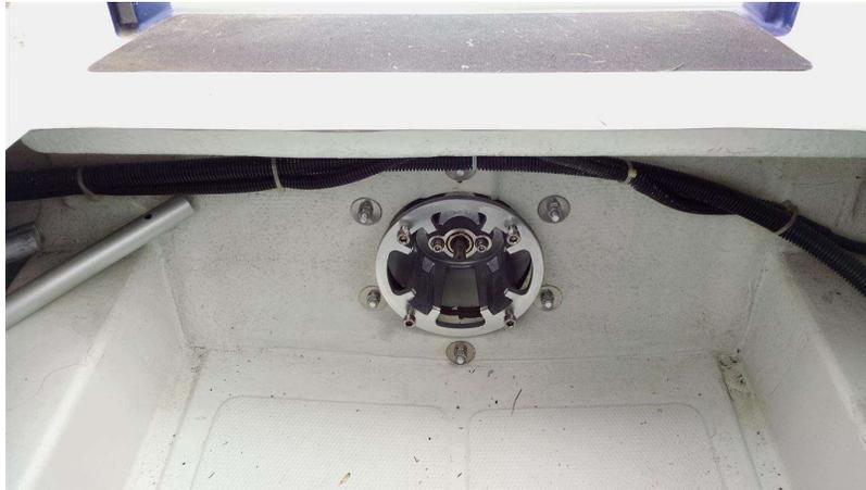
The next step is to mount the motor to the bracket. The manual says the motor needs to be supported from underneath so that the tunnel bracket doesn't take the load of the 30lb motor. I wrestled with this for quite a while, as they described glassing in a wood beam underneath, etc. I didn't want to mess with all that.
