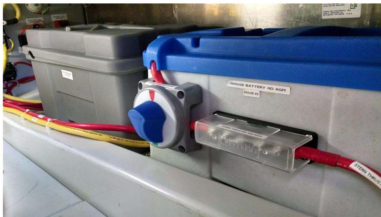
This is the 3<sup>rd</sup> house battery that was added. The main engine start battery is ahead of it now. You can see the positive lead from the switch going into the house bank battery to do its business. The red and yellow coming around the side are tying into the other two.
