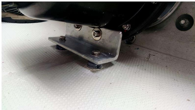
At this point the motor appeared to be well supported and felt really rigid.
