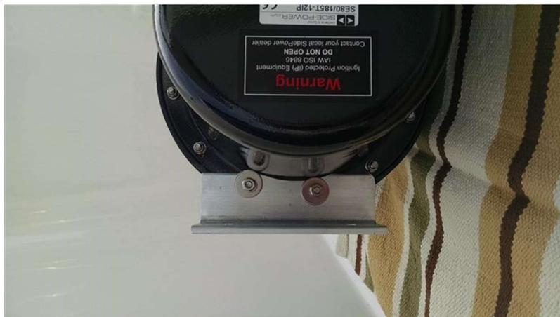
Next, I mounted the motor, measured, and marked the floor about 6 (no, maybe 8) times. Then I epoxied two 10-24, 316 stainless threaded inserts into the floor, aligned with the holes in the aluminum angle.
