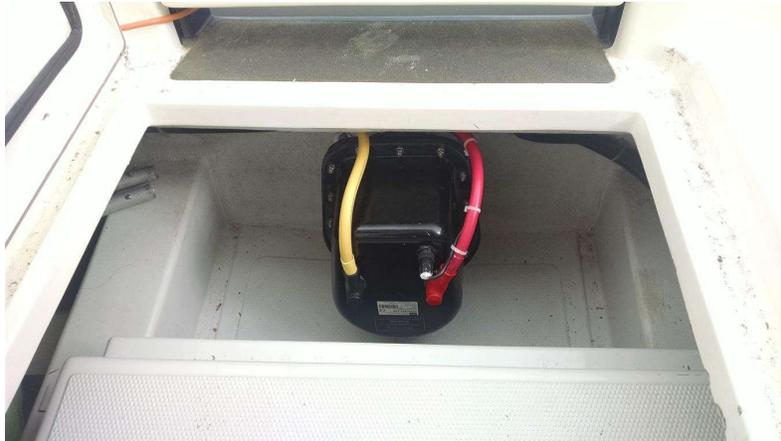
I came down the side of the freshwater tank on the sole and connected up to the aft-most house battery (of 3). I couldn't find a good place to mount the emergency cutoff switch and fuse block, so I took the battery out and bolted them right to the battery box!
