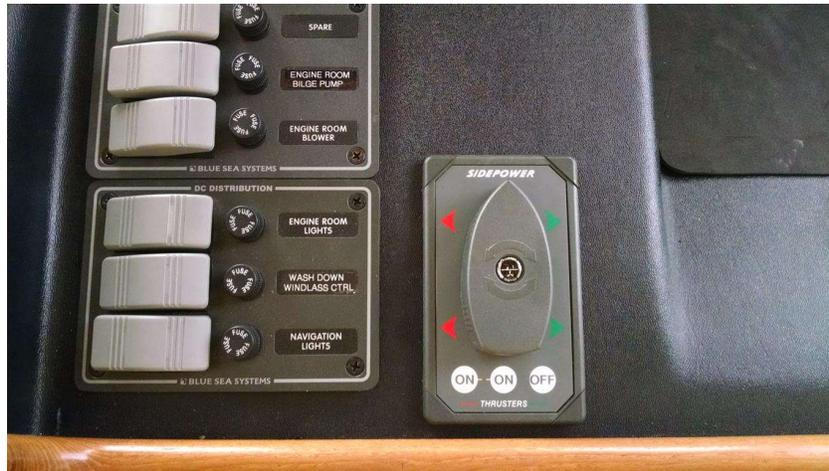
Last step was the wireless control install. I put the transceiver behind the steering panel at the helm. All of the control cabling was plug and play. I did have to pull the contacts out of one of the connectors to snake everything through all the holes and then put them back for final connection. Here is the wireless remote ready for action!
