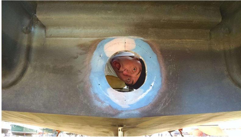
I coated all of the sanding and the edges of the holes with several coats of epoxy.
