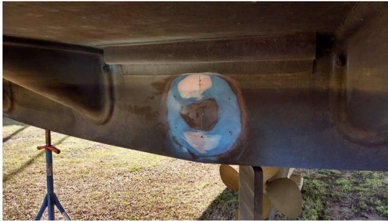
Next, out came the jigsaw. Beware of the hydraulic lines inside the lazarette, and be aware how thick the hull bottom is in order for the lowest bolt to come through "above ground".
