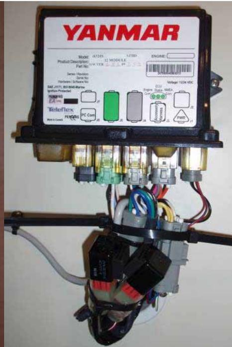
*Install the harness in-between engine harness and i832X module*
