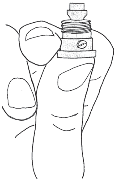
Figure 37. Checking Delivery Valve.
