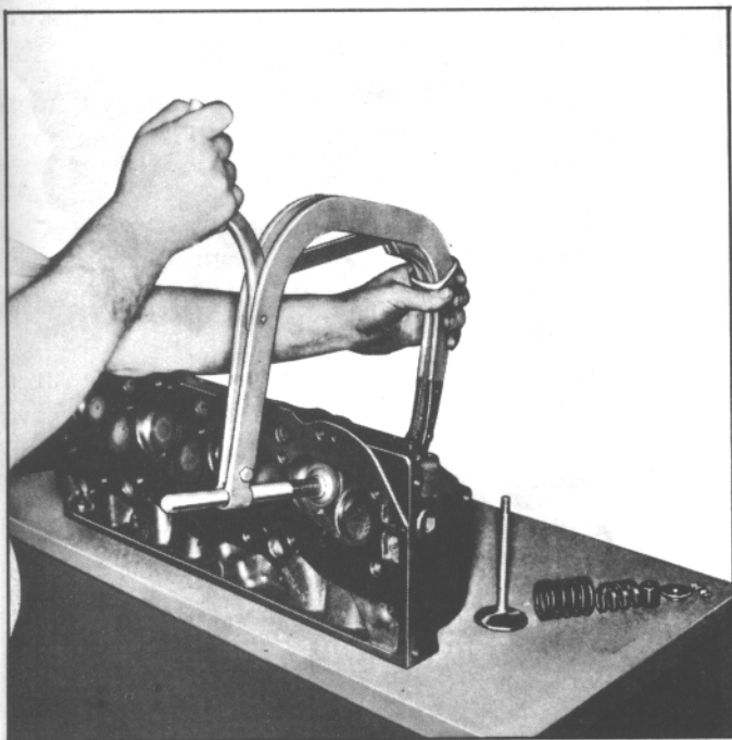
Fig. 96. Compressing Valve Spring
