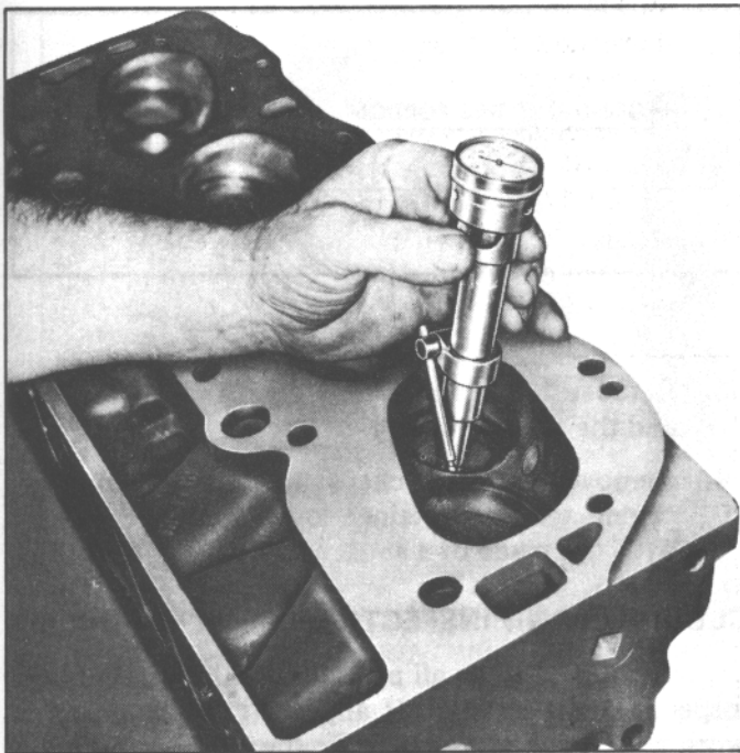
Fig. 107. Measuring Valve Seat Concentricity
