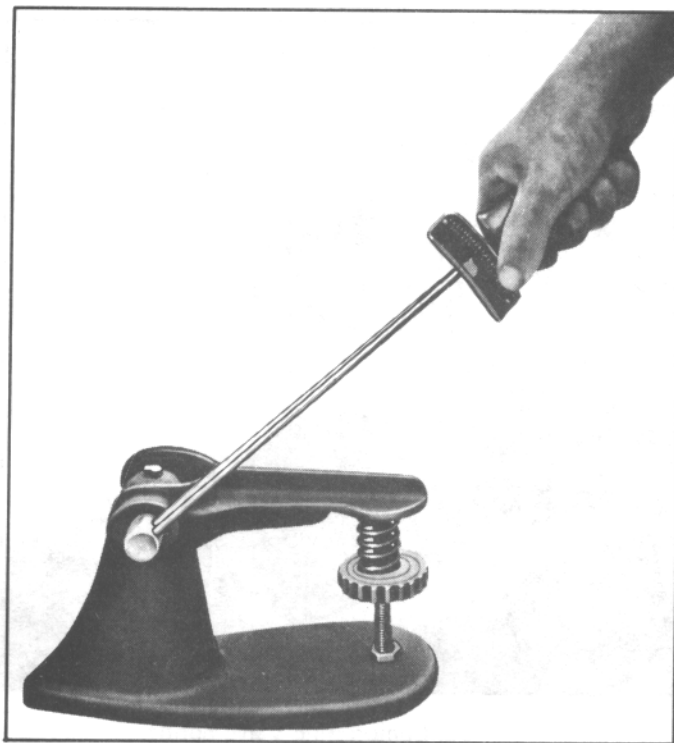
Fig. 100. Checking Valve Spring Tension
