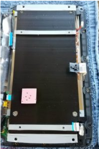
Heat sink with insulator pad
