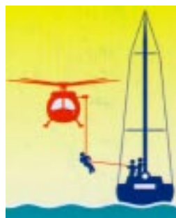
The NEST hi-line technique, in this case shown with a vessel with rigging intact.
