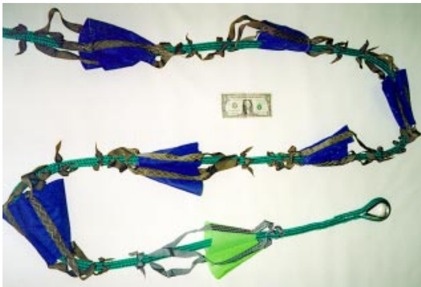
The Jordan series drogue consists of numerous small elements, each of which contributes a modest amount of drag; the aggregate of which is an enormous braking power.
