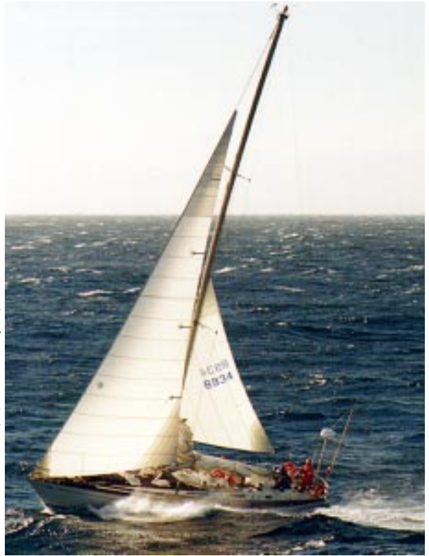
Here is a moderate gale combination: a full-sized number-4 jib together with trysail. A deeply reefed main could be flown in lieu of the trysail. However, this would subject the main to extra stress. With the trysail set in moderate conditions you are ready for the weather to get worse.
