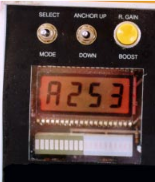
The "gain boost" button in the upper right corner is a key feature in the WH Storm Pilot operation. When you hit this button with your thumb it doubles rudder gain, cranking in twice as much course correction as normally used. This helps to pull the bow down quickly when you are slapped by a wave on the stern and start to round up. Once the rudder has a good grip, lift your thumb and gain returns to the normal setting, avoiding the problem of overshooting the course and sailing by the lee (or accidentally jibing).
