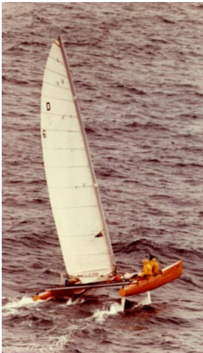
Beowulf V powered up and out ahead of the "official" fleet. We would normally be sailing from double trapezes, but offshore like this, we stayed on the hull to reduce structural loading on the beams and hulls.
