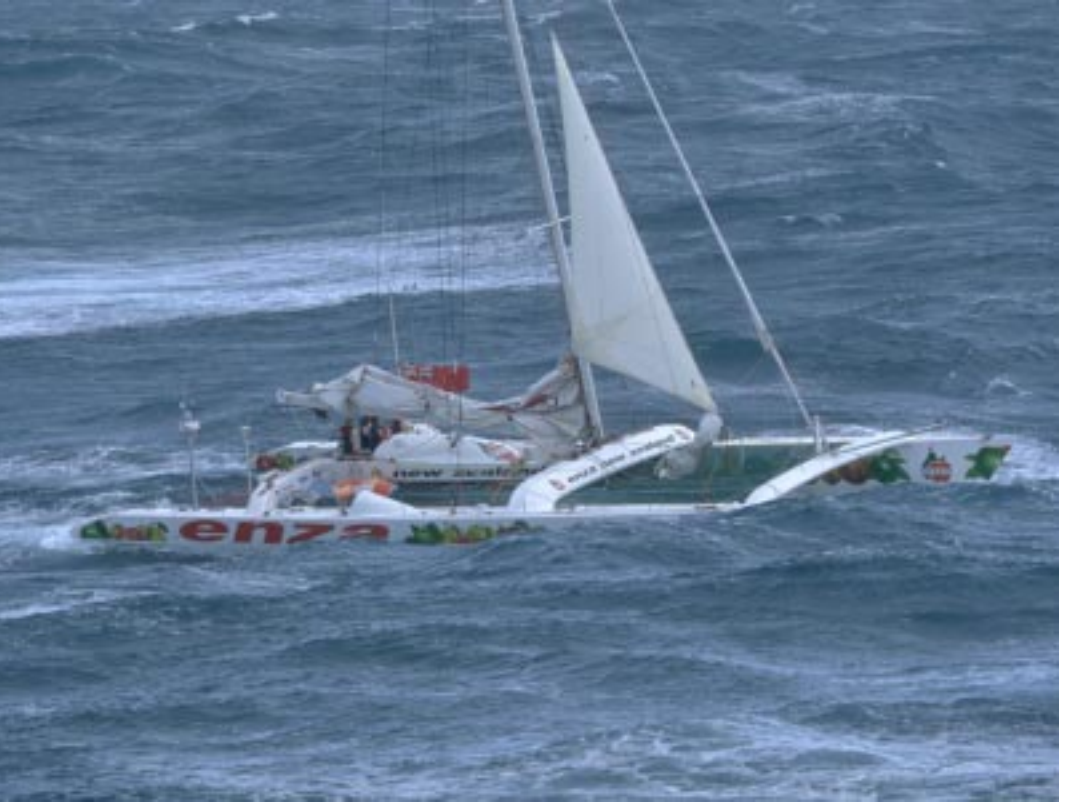
The 80-foot (24.5m) catamaran Enza at the finish of her circumnavigation. The winds are storm force and above, seas are short and breaking. This is a huge, powerful multihull, being sailed by some of the best seamen on the planet. Note the tiny storm jib set on the cutter stay. Enza is also towing all of the extra rope and chain they have aboard to try to slow progress.
