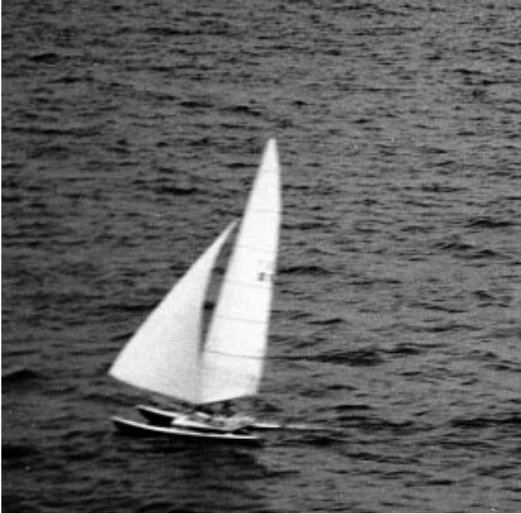
The Hobie Super 16 en route to Ensenada. Check out the rig— 32-foot (10m) tall mast (on a 16-foot/5m boat!), 180-square-foot reacher, and a huge main-sail. To sail this boat through the gale and keep it afloat was an amazing feat.
