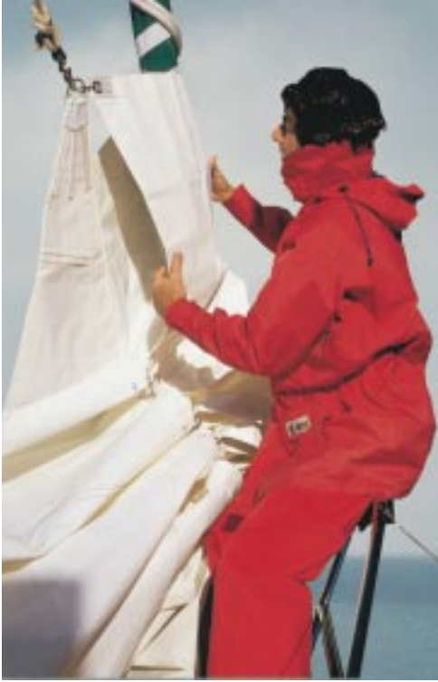
The Gale Sail attaches around the roller-furled headsail. The ideal time to set this sail is well before it is needed, by running off dead downwind and keeping the sail in the lee of the mainsail.
