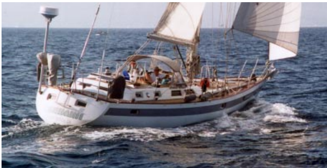
Shakti is 44 feet 7 inches (13.7m) long, 39 feet (12m) at the waterline, with a beam of 13 feet (4m) and draft of 6 feet 6 inches (2m). As cruising boats go, she's relatively quick.
